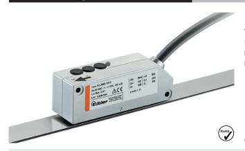
The non-contact absolute magnetic linear measurement system Limes LA50 / BA5 - made up of the sensor head LA50 and of the magnetic band BA5 - reaches a resolution up to 10  $\mu$ m with a maximum distance of 1.5 mm between the sensor and the band.
