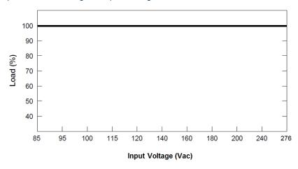
No output power de-rating for the input voltage range
