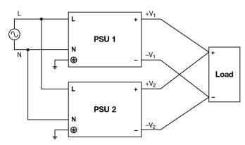
Fig. 9 Redundant & Parallel Operation Connection Diagram
